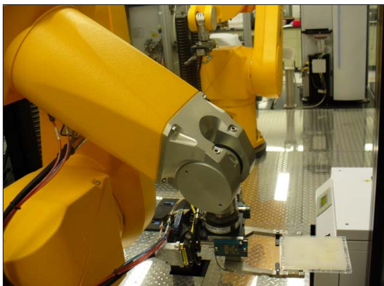
A robot at the NIH Chemical Genomics Center (NCGC) holds a 1,536 well plate similar to the ones to be used in the STAR high-throughput screening.
